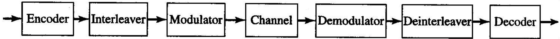
Figure 9.19 Block diagram of a system that employs interleaving/deinterleaving for burst-error-correction.
