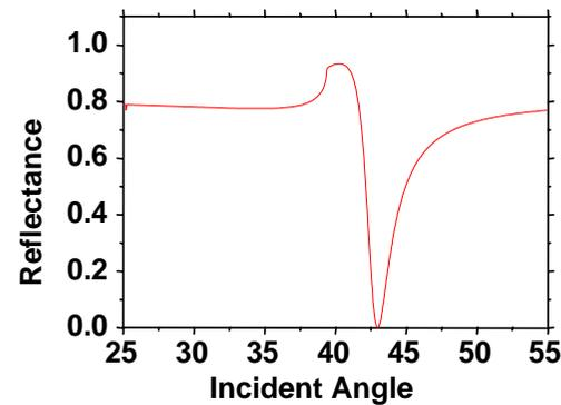
**Binding causes the dip to shift.**
