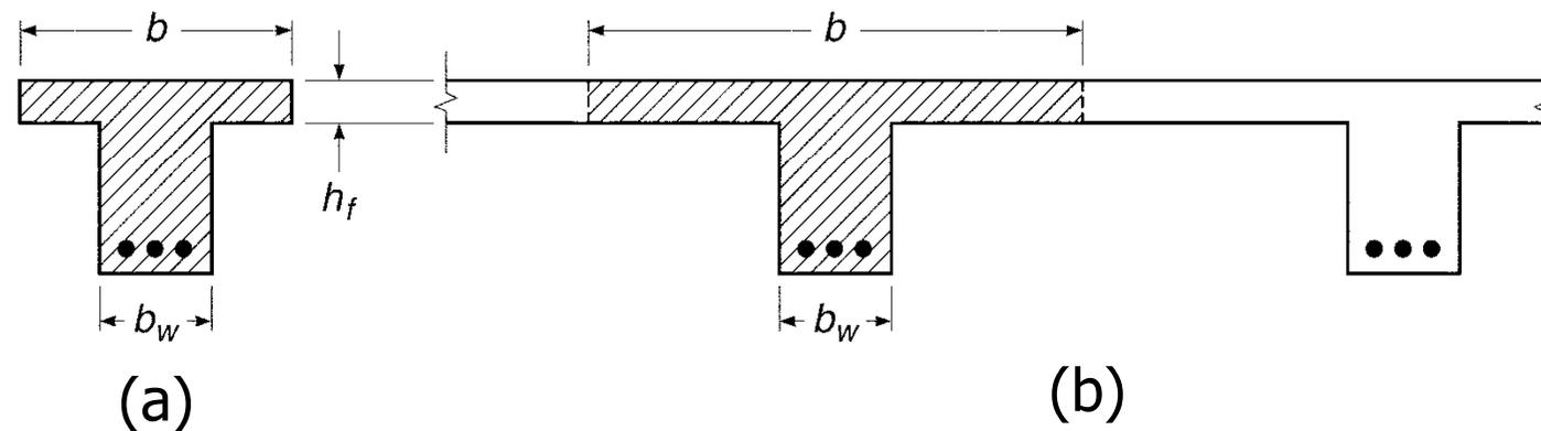
In (b) of the above figure, the element of the flange between the webs are **less stressed** than the element directly over the web due to the effect of SHEAR deformation of the flange.
