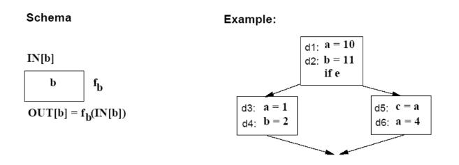
\* A transfer function  $f_b$  for a basic block *b*:  $OUT[b] = f_b(IN[b])$
