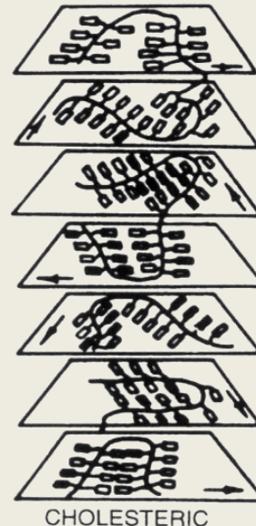
Fig. 7.7 A schematic showing how mesogenic LC side-chain polymers can be organized into different mesophases.
