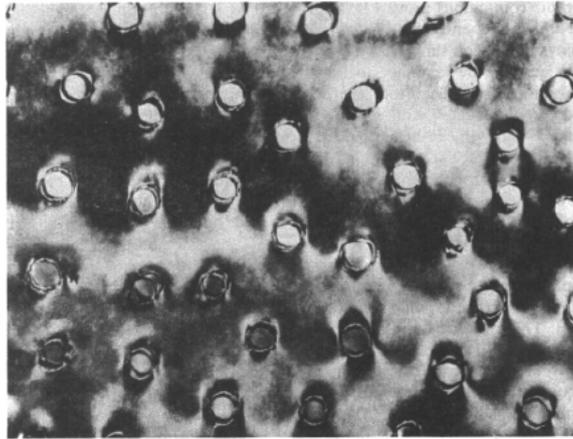
**Fig. 4.30** Rod-like eutectic. Al<sub>6</sub>Fe rods in Al matrix. Transverse section. Transmission electron micrograph (× 70000). (Courtesy of J. Strid, University of Lulea, Sweden.)
