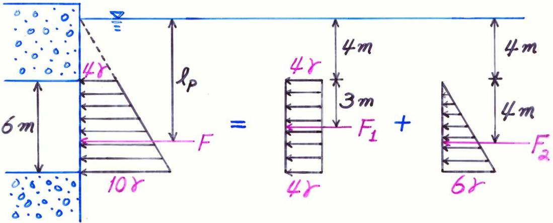
$$\left. \begin{array}{l} F_1 = 4\gamma \times (6 \times 8) = 192\gamma \\ F_2 = \frac{6\gamma \times 6}{2} \times 8 = 144\gamma \end{array} \right\} \rightarrow F = F_1 + F_2 = 336\gamma$$
