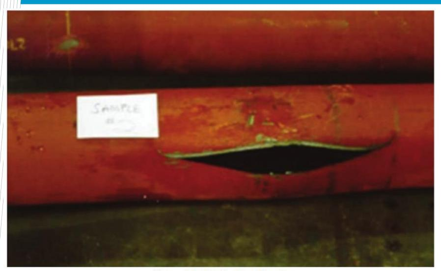
Figure A.1—Ductile Burst Sample
