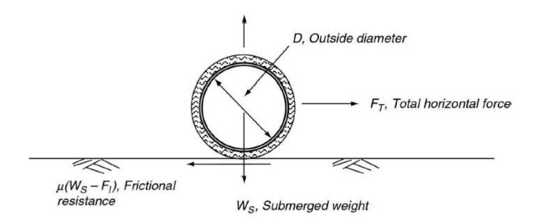
FIGURE 13.1 Forces acting on the pipeline resting on the seabed.
