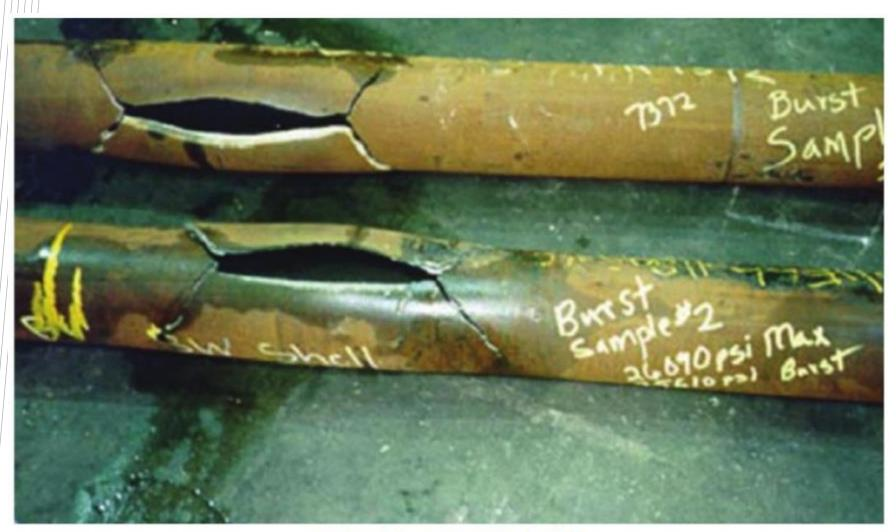
Figure A.2—Brittle Burst Sample
