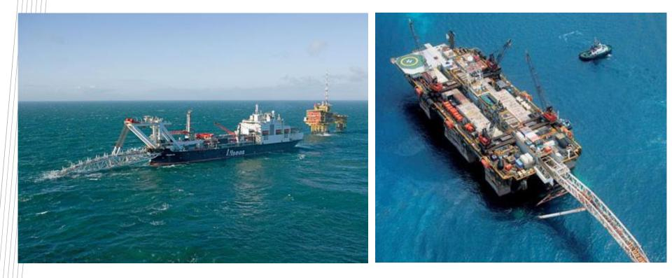
• Pipeline Installation Vessel (J-Lay)
