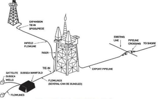
Figure 27-1 Application of Subsea Pipelines
