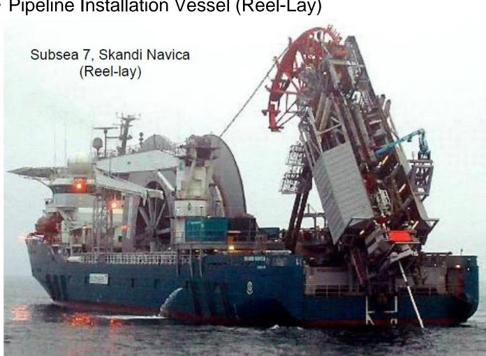
• Pipeline Installation Vessel (Reel-Lay)
