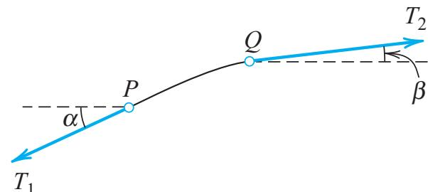
$$\Rightarrow \frac{T_2 \sin \beta}{T_2 \cos \beta} - \frac{T_1 \sin \alpha}{T_1 \cos \alpha} = \frac{\rho}{T} \Delta x u_{tt} \Rightarrow \tan \beta - \tan \alpha = \frac{\rho}{T} \Delta x u_{tt}$$
