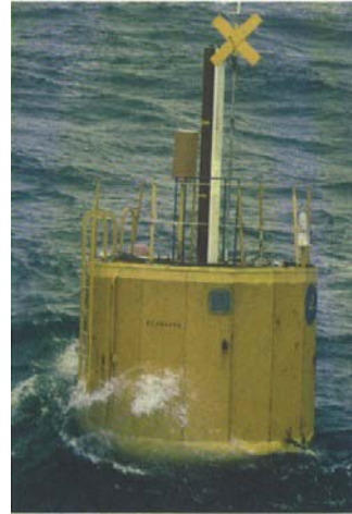
Figure 8.25 The AquaBuoy system, based on the IPS and hose pump concepts
