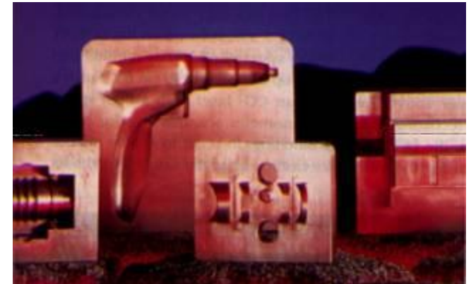
Core and cavity sets produced by RapidTool™
