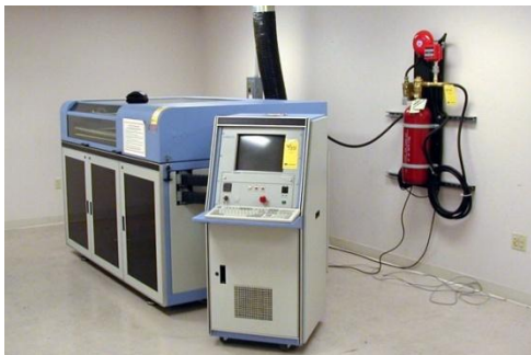
Helisy 2030E LOM machine Part envelope size 32"x22"x20"
