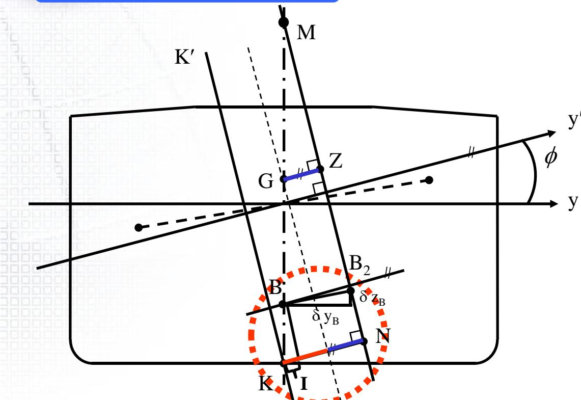
$$\begin{aligned} \mathbf{KN}(\phi) &= I + II + III \\ &= \mathbf{KB} \sin \phi + \delta y_B \cos \phi + \delta z_B \sin \phi \\ &= \mathbf{KG} \sin \phi + \mathbf{GZ} \end{aligned}$$
