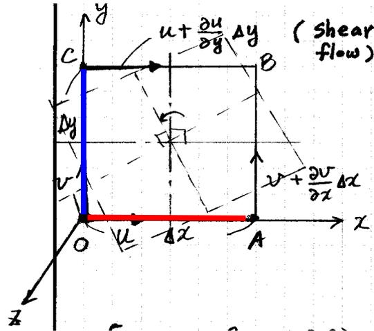
Assume the rate of rotation of fluid element  $\Delta x$  and  $\Delta y$  about  $z$ -axis is positive when rotate counterclockwise.
