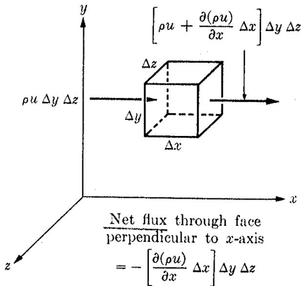
Consider differential (infinitesimal) control volume ( $\Delta x \Delta y \Delta z$ )
