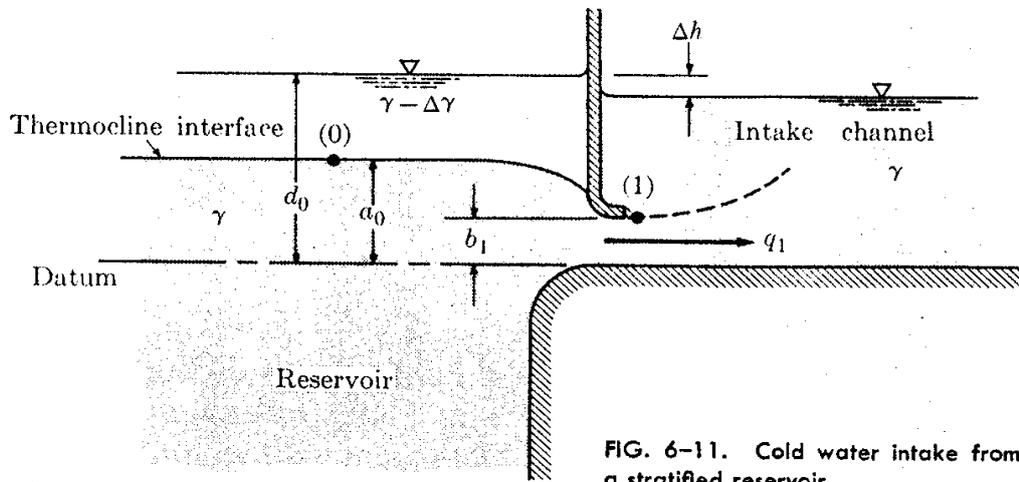
FIG. 6-11. Cold water intake from a stratified reservoir.
