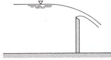
FIG. 6-9. Flow over a weir under gravity forces.
