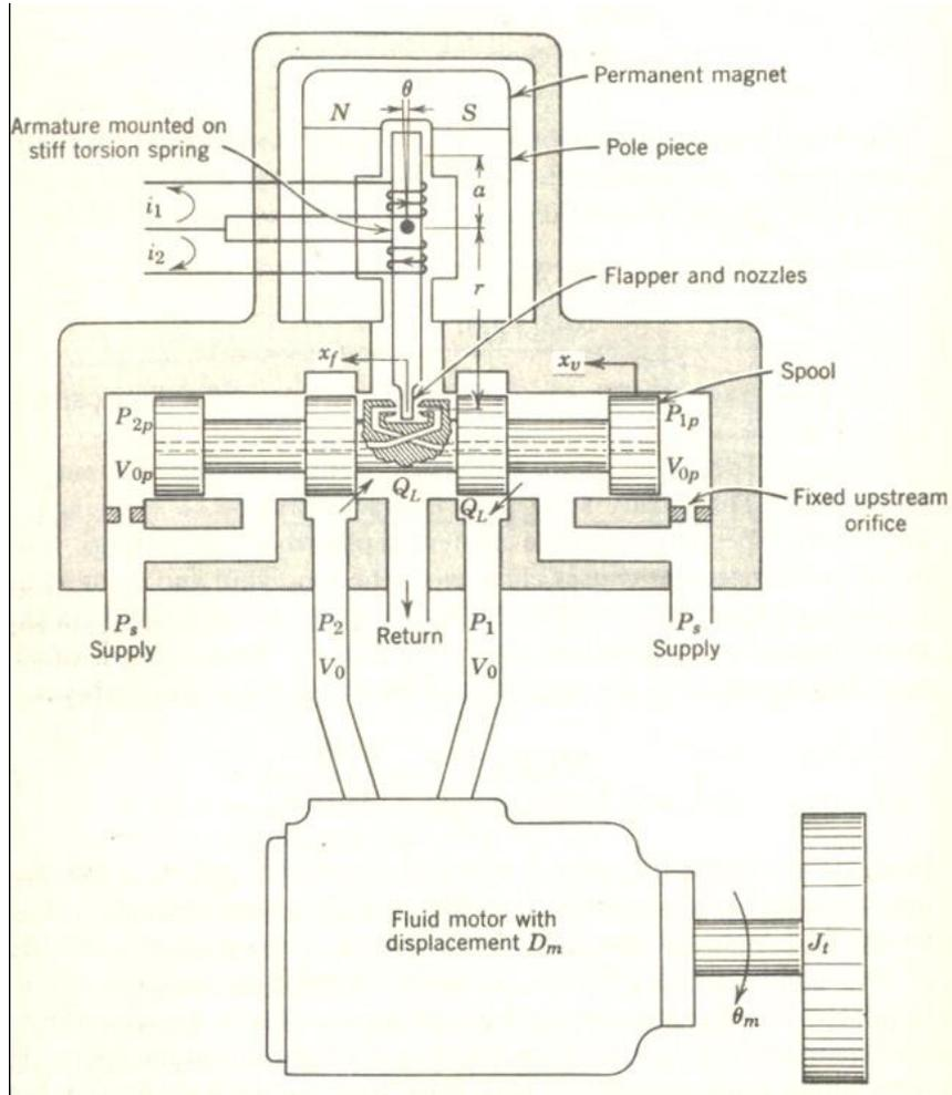
Schematic of a two-stage electrohydraulic servovalve with force feedback controlling a motor with inertia load
