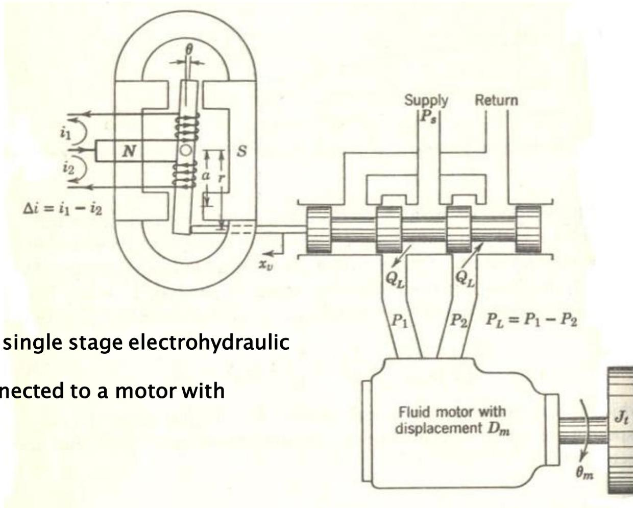
Schematic of a single stage electrohydraulic servovalve connected to a motor with inertia load
