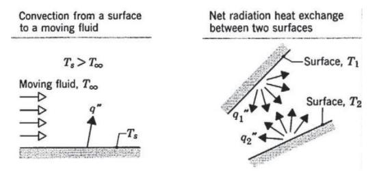
Although these three heat transfer modes occur at all subsea systems, for typical pipelines, heat transfer from radiation is relatively insignificant compared with heat transfer from conduction and convection.
