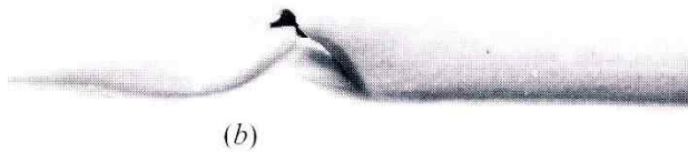
Aluminum alloy tube (brittle): compressive failure
