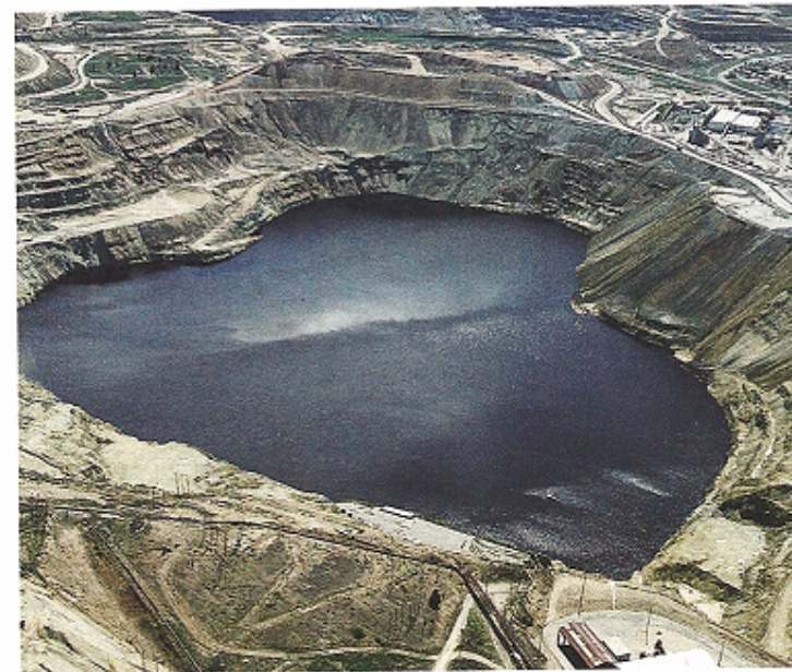
Figure 14.12 Closed mine filling with toxic water The Berkeley Pit near Butte, Montana, a polluted lake in a closed copper mine. (Calvin Larsen/Photo Researchers, Inc.)
