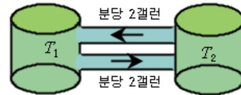
$y_1(t)$ : amount of fertilizer in  $T_1$ ,  $y_2(t)$ : amount of fertilizer in  $T_2$
