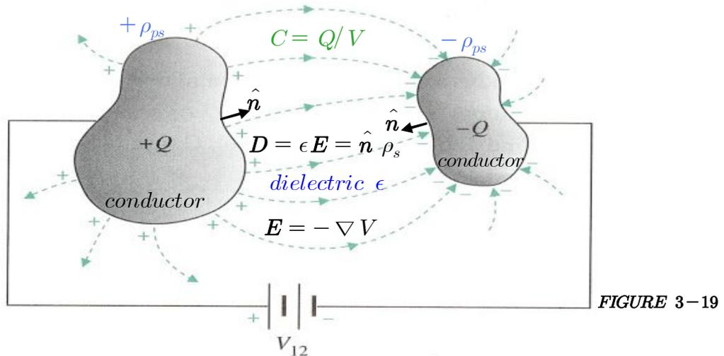
**Capacitor** = a device for storing electric charge (i.e., electric energy) consisting of two conductors separated by a dielectric
