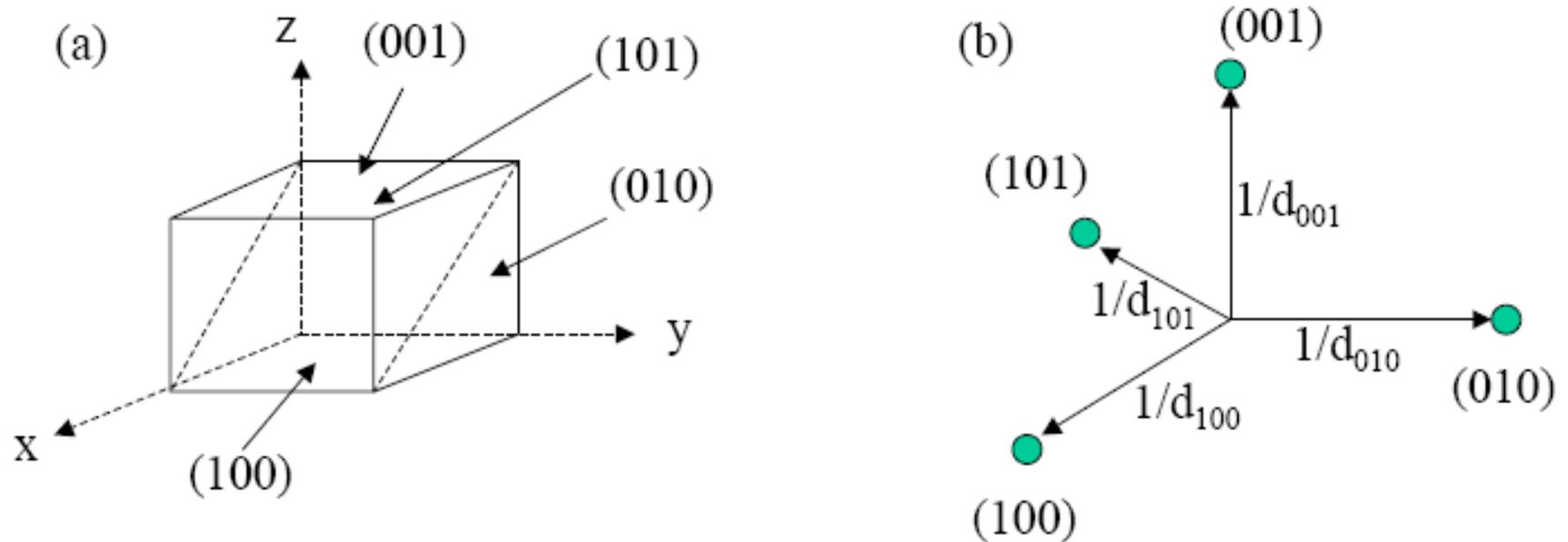
Figure (a) The relationship between crystal planes. (b) The relationship between equivalent reciprocal lattice points
