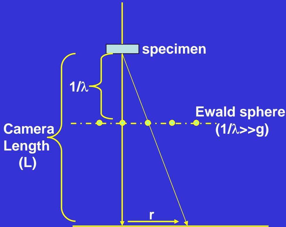
The single crystal electron diffraction pattern is a series of spots equivalent to a magnified view of a planar section through the reciprocal lattice normal to the incident beam.
