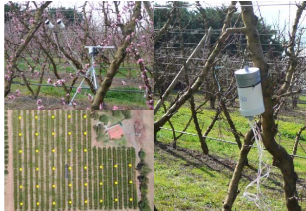
Soil moisture sensor nodes
