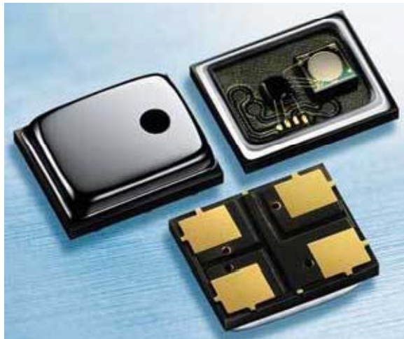
Silicon microphone (Knowles Acoustics)
