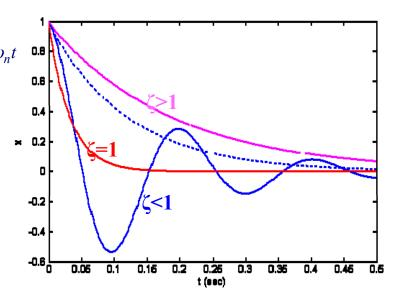
Where  $\omega_d = \omega_n \sqrt{1 - \zeta^2} = \text{damped natural frequency}$
