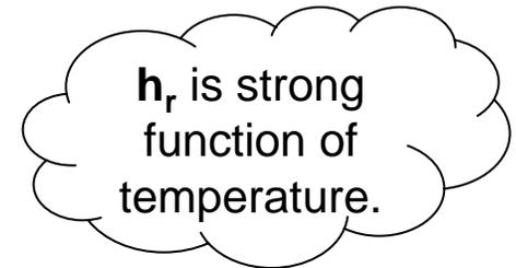
$$h_r = \sigma(T_1^3 + T_1^2 T_2 + T_1 T_2^2 + T_2^3) \quad (26-35)$$
