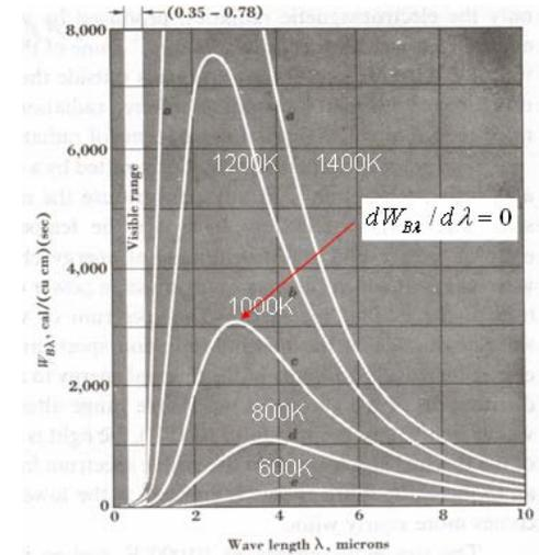
A decreasing wavelength at peak emissive power for increasing temperature.
