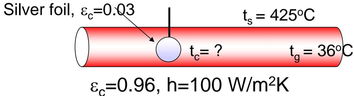
(b) If silver foil is wrapped, what will be the new thermometer reading?
