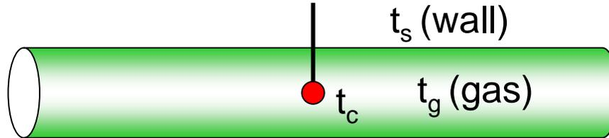
A thermocouple used to measure a fluid temperature in a container may give a reading significantly different from the fluid temperature **if the walls are at some other temperature.**
