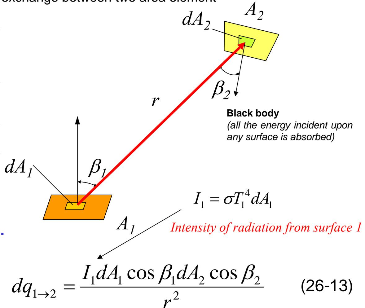
The rate of transfer of radiant heat from 1 to 2
