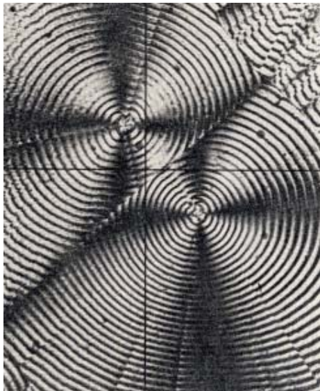
Figure 21 Two impinging banded spherulites between crossed polarizers
