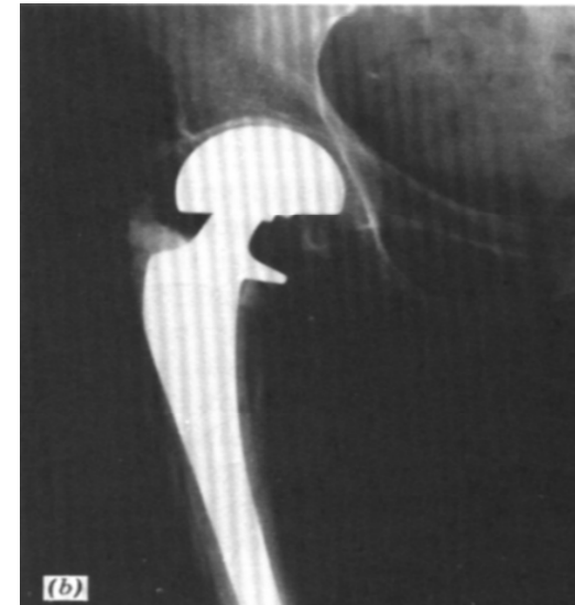
Hip implant-cyclic loading from walking
