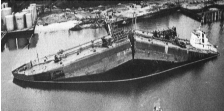
Ship-cyclic loading from waves
