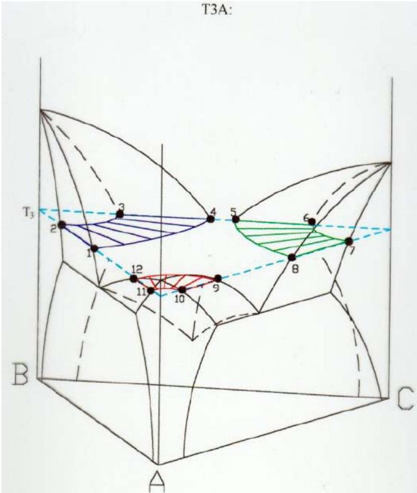
Temperature Slice At  $T_3 < T_A, T_B, T_C$ , But  $T_3 > T_{E1}, T_{E2}, T_{E3}$
