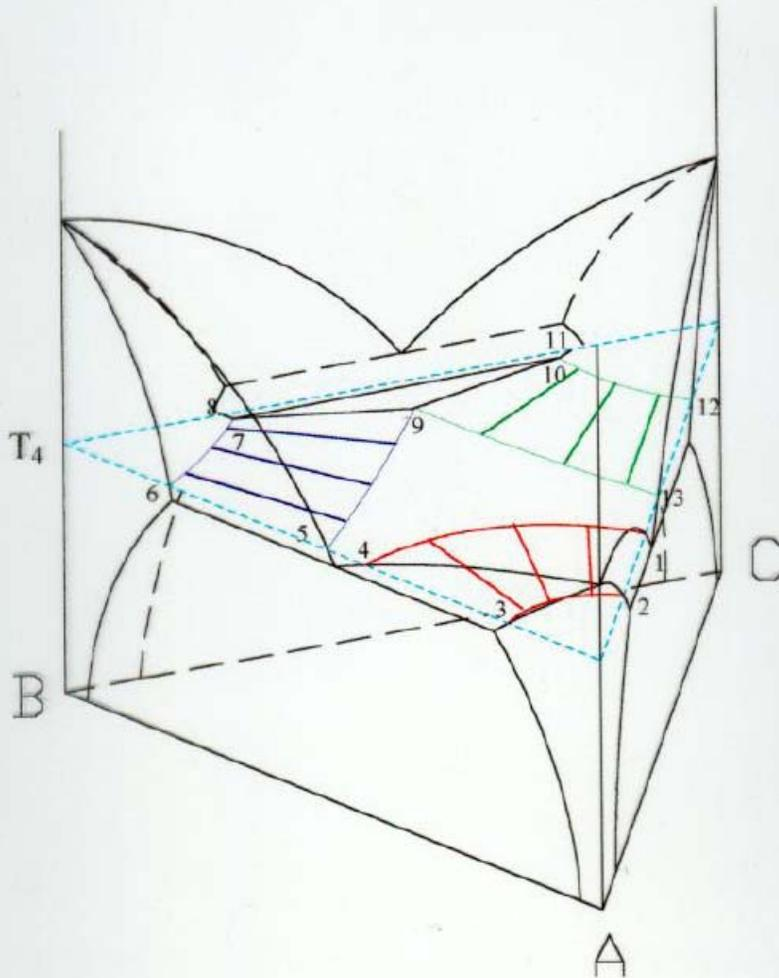
Temperature Slice At  $T_4 < T_{E2}$  And  $T_4 > T_{E1}, T_{E3}$
