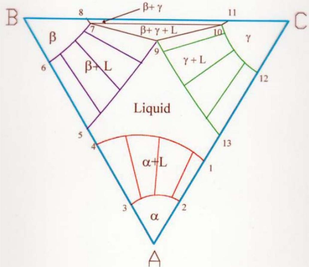
Isothermal Section At  $T = T_4$
