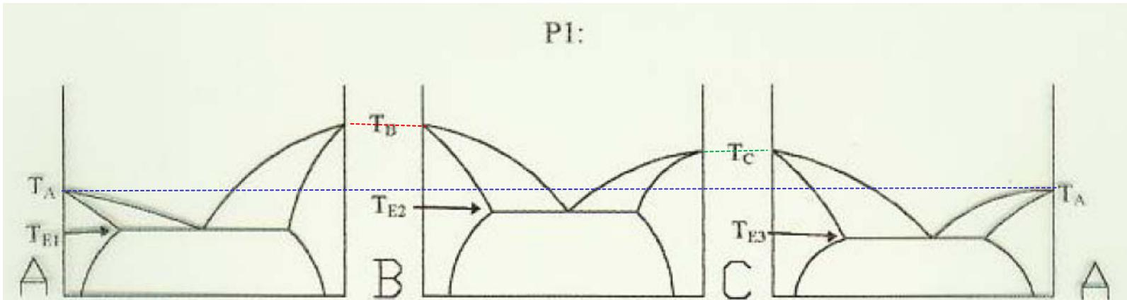
$T_A$ : Melting Point Of Material A
