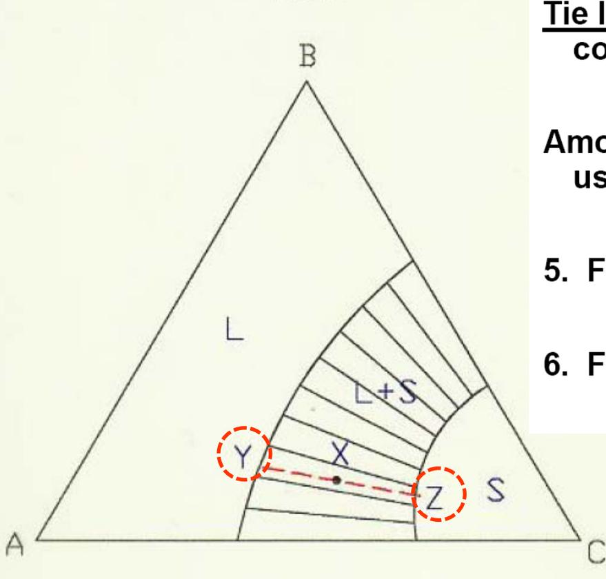
**Tie line**: A straight line joining any two ternary compositions
