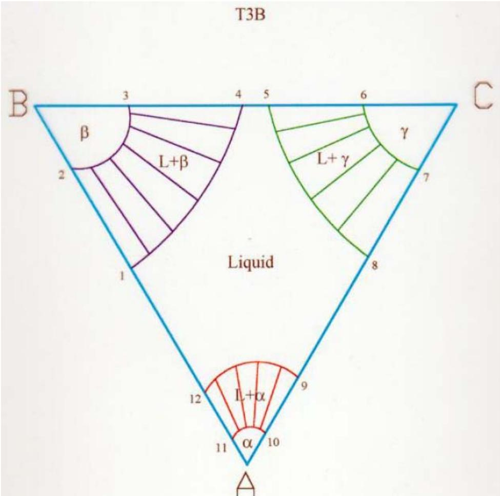
Isothermal Section At  $T = T_3$
