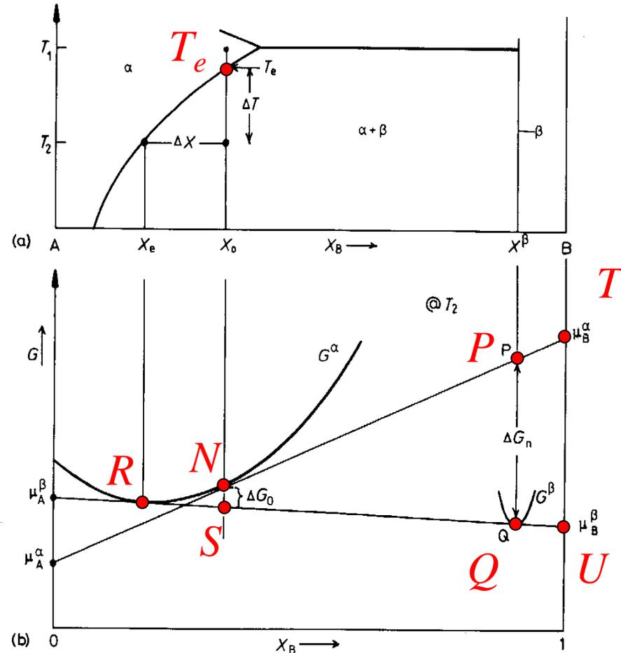
Fig. 5.3 Free energy changes during precipitation. The driving force for the first precipitates to nucleate is  $\Delta G_n = \Delta G_V V_m$ .  $\Delta G_0$  is the total decrease in free energy when precipitation is complete and equilibrium has been reached.
