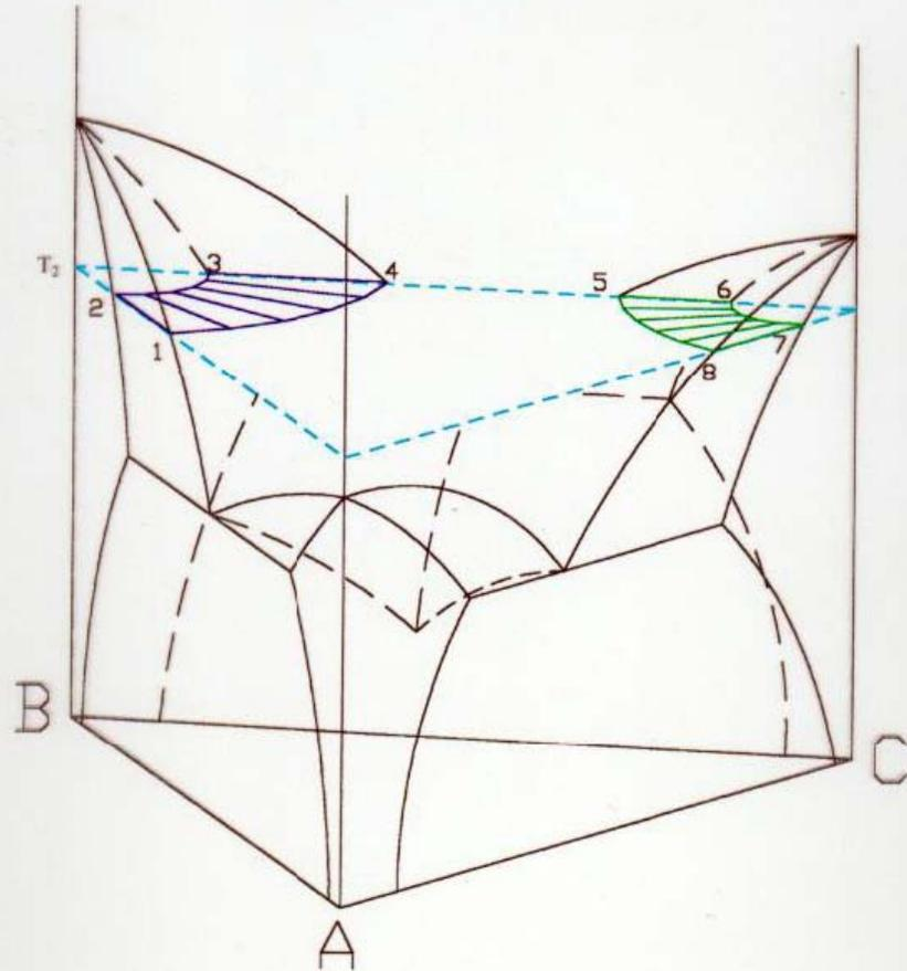
Temperature Slice At  $T_2 > T_A$  But,  $T_2 < T_B, T_C$
