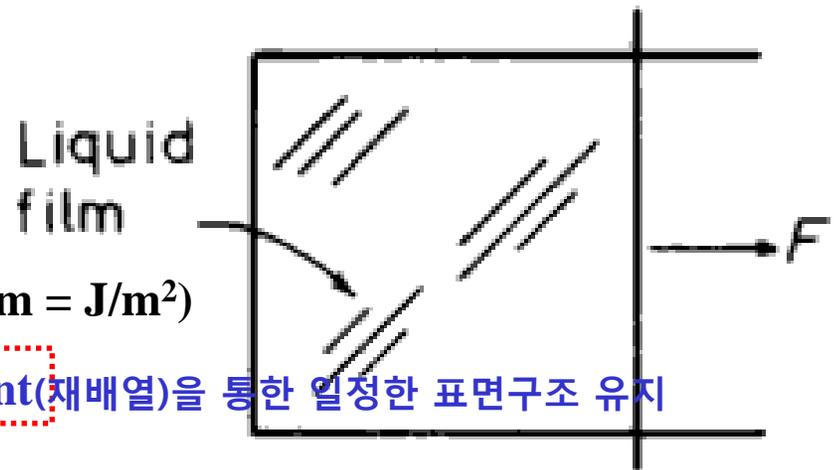
Fig. 3.1 A liquid film on a wire frame.
