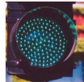
Fig. 1.12. Green traffic signals are one of the ubiquitous applications of GaInN/GaN green LEDs.
