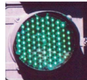
Fig. 1.12. Green traffic signals are one of the ubiquitous applications of GaInN/GaN green LEDs.
