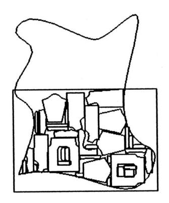
Nesting of 36 patterns on an irregular raw sheet with an interior defect
