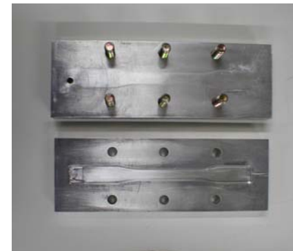
Two-part mold for injection molding
