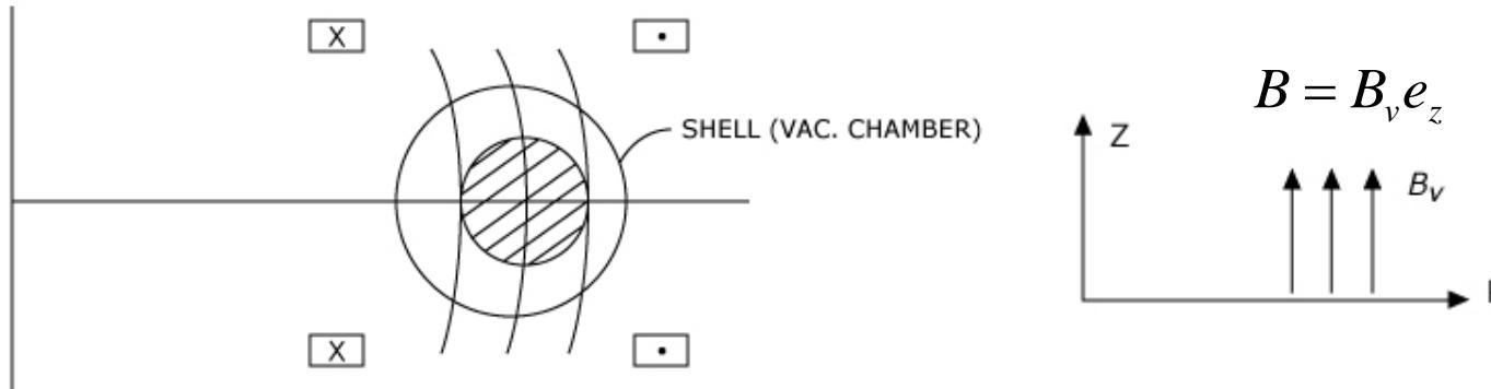
The vertical field causes a shift of the plasma surface with respect to  $R_0$ .
