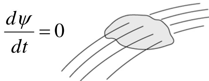
time rate of change of the flux passing through any moving surface,  $S$
