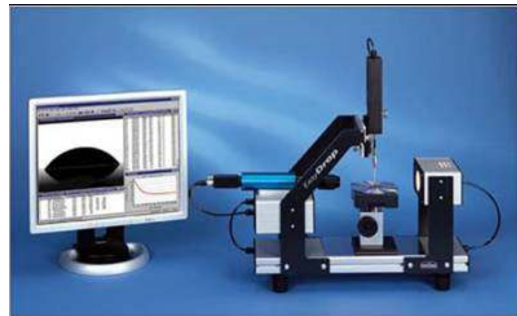
Goniometer for measuring contact angle
