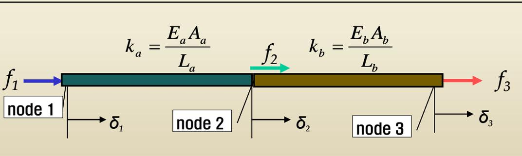
$$\begin{bmatrix} f_1 \\ f_2 \\ f_3 \end{bmatrix} = \begin{bmatrix} \frac{E_a A_a}{L_a} & -\frac{E_a A_a}{L_a} & 0 \\ -\frac{E_a A_a}{L_a} & \frac{E_a A_a}{L_a} & 0 \\ 0 & 0 & 0 \end{bmatrix} + \begin{bmatrix} 0 & 0 & 0 \\ 0 & \frac{E_b A_b}{L_b} & -\frac{E_b A_b}{L_b} \\ 0 & -\frac{E_b A_b}{L_b} & \frac{E_b A_b}{L_b} \end{bmatrix} \begin{bmatrix} \delta_1 \\ \delta_2 \\ \delta_3 \end{bmatrix}$$
