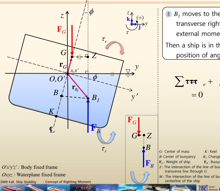
(8)  $B_1$  moves to the right side until transverse righting moment and external moment are balanced. Then a ship is in the static equilibrium at position of angle  $\phi$  of heel
