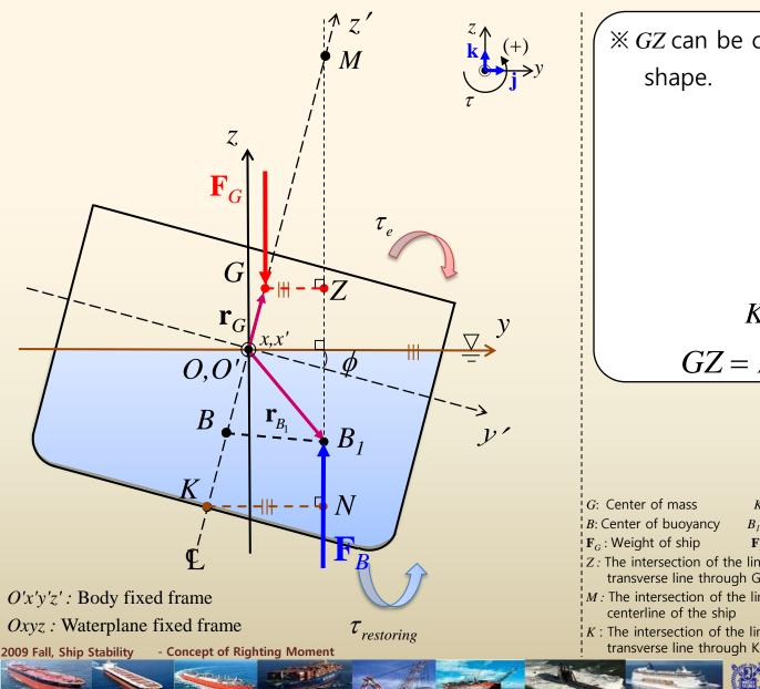
※ GZ can be calculated in geometrical shape. M \_\_\_\_₩  $GZ = KN - KG \sin \phi$
