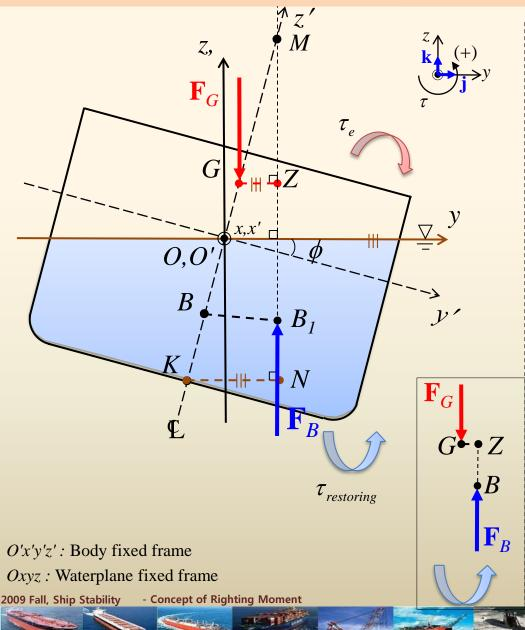
• **Righting Moment :** Moment to return the ship to the upright floating position (Moment of statical stability))
