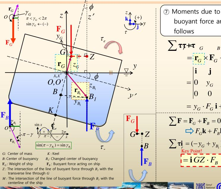
⑦ Moments due to weight of ship and buoyant force are calculated as follows
