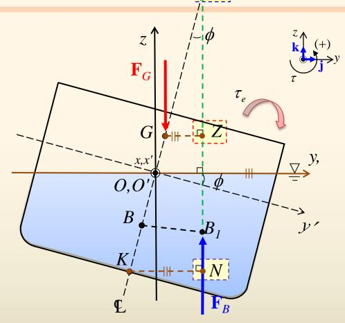
*O'x'y'z'* : Body fixed frame *Oxyz* : Waterplane fixed frame 2009 Fall, Ship Stability - Concept of Righting Moment ⑥ Define M, Z, N which is based on the vertical line through heeled center of buoyancy
