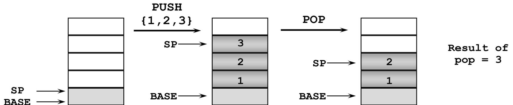
⌘ Traditionally, a stack grows down in memory, with the last “pushed” value at the lowest address. The ARM also supports ascending stacks, where the stack structure grows up through memory.
