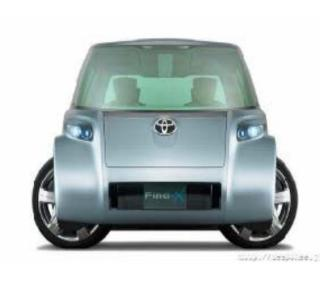
4Wheel independent drive 4wheel independent steering 4wheel independent braking By 'wheel-in-motor'
