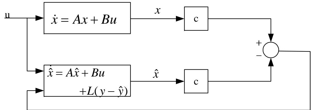
$$\begin{aligned}\dot{\hat{x}} &= A\hat{x} + Bu + L(cx - c\hat{x}) = (A - LC)\hat{x} + Bu + LCx \\ \dot{e} &= (A - LC)e\end{aligned}$$
