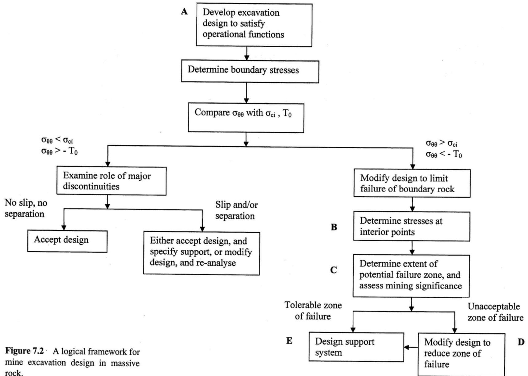
**Figure 7.2** A logical framework for mine excavation design in massive rock.
