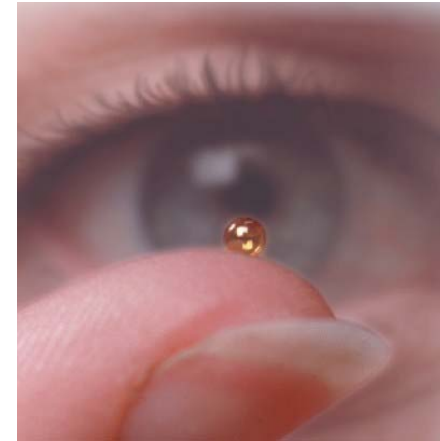
Image of an inertial confinement fusion fuel microcapsule. Taken from LLNL Sep. 2002 ST&R publication.
