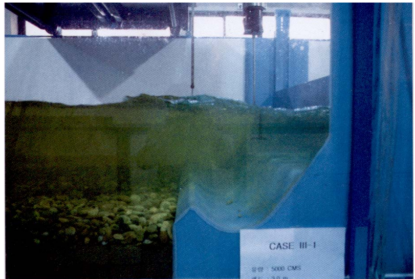
Jamshil submerged weir Model Test ( Q = 5,000 \text{ m}^3/\text{s} )
