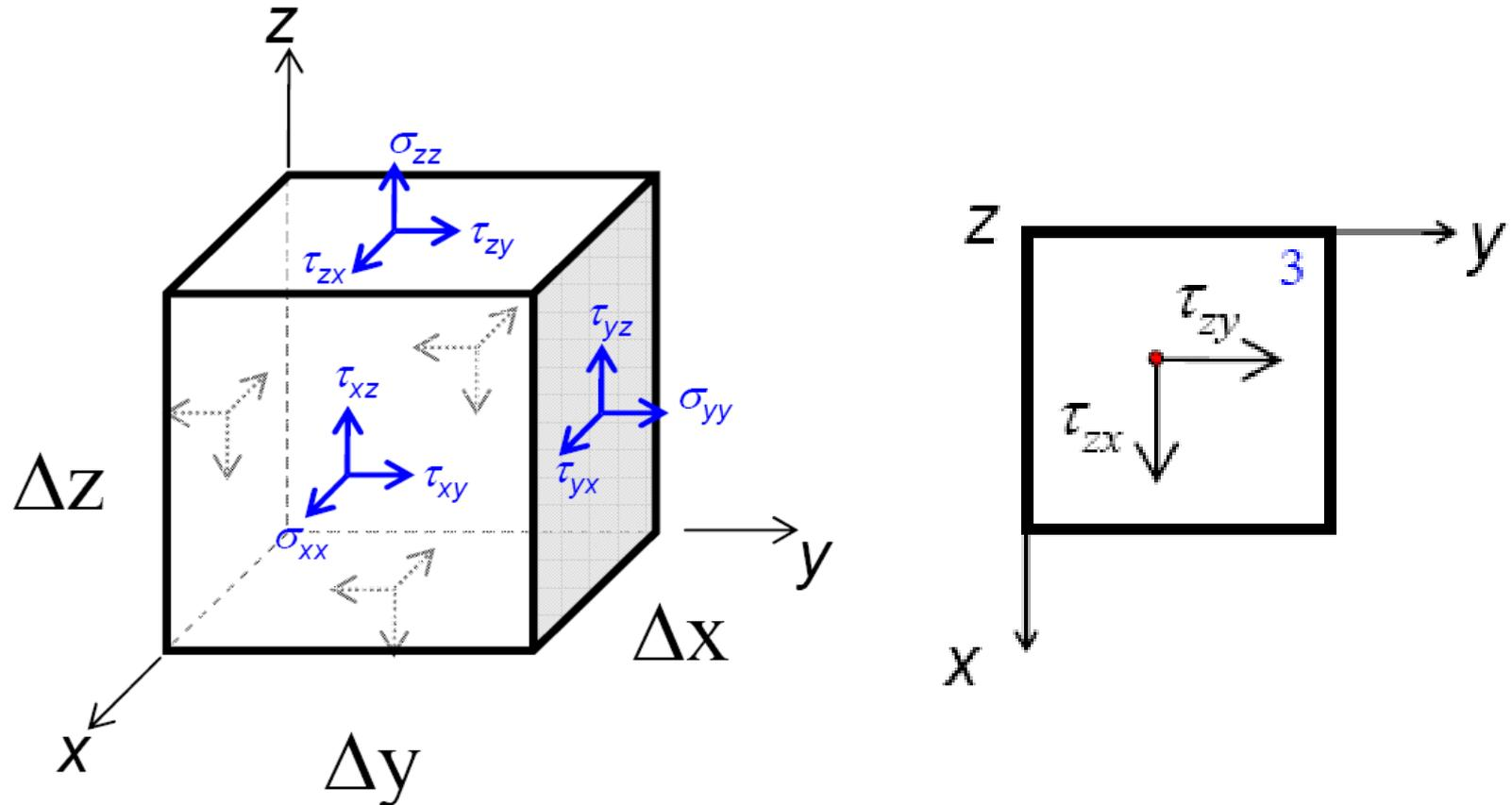
This construction automatically implies **the need for 18 stress components to define the state of stress** in the volume element.
