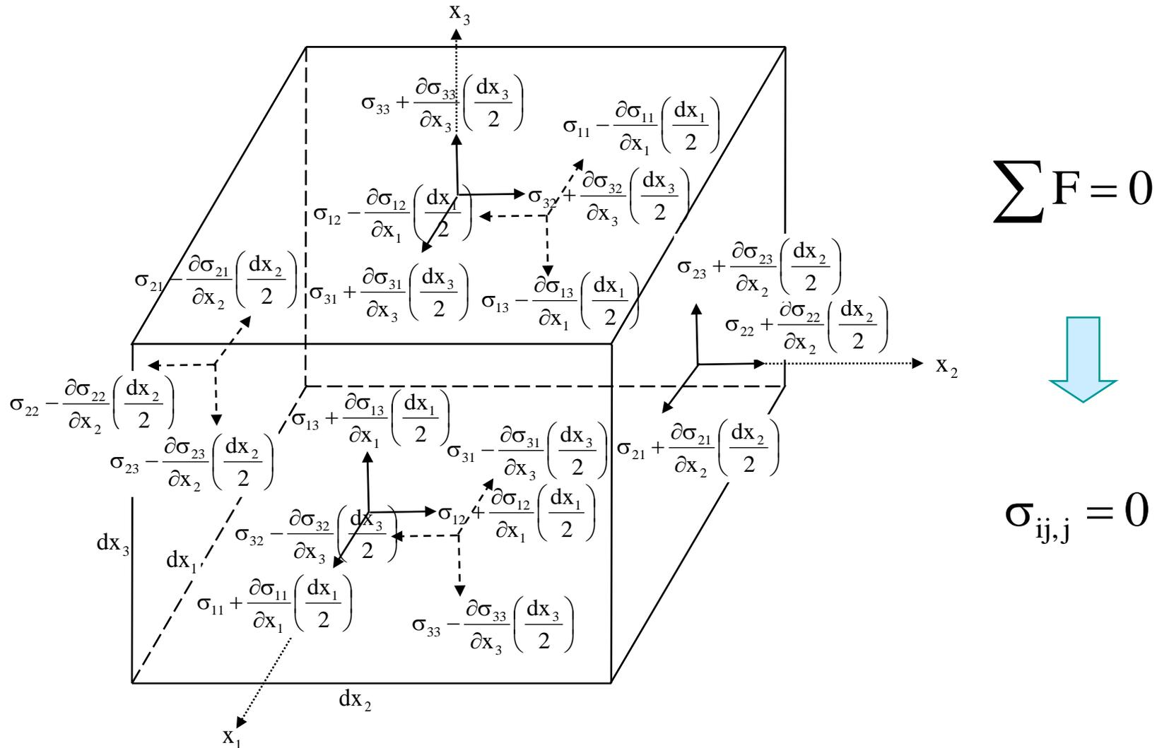
Stress distribution in an infinitesimal element
