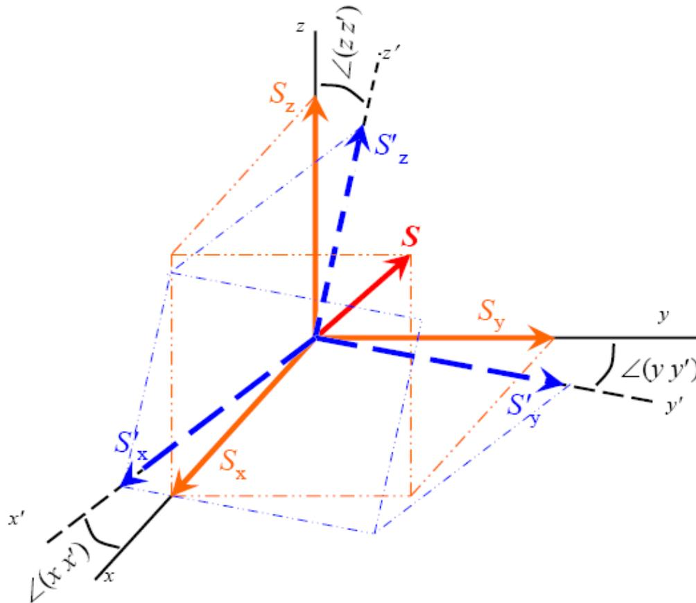
**The vector  $S$  can be easily resolved into components that are parallel to any set of reference axes.**
