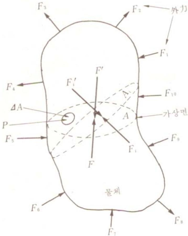
The forces acting within a stressed body are either body forces or surface forces.
