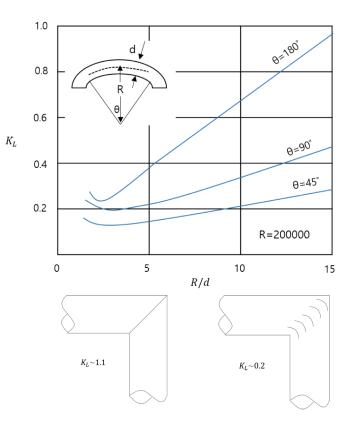
Miter fit needs to special design for breaking stream line
