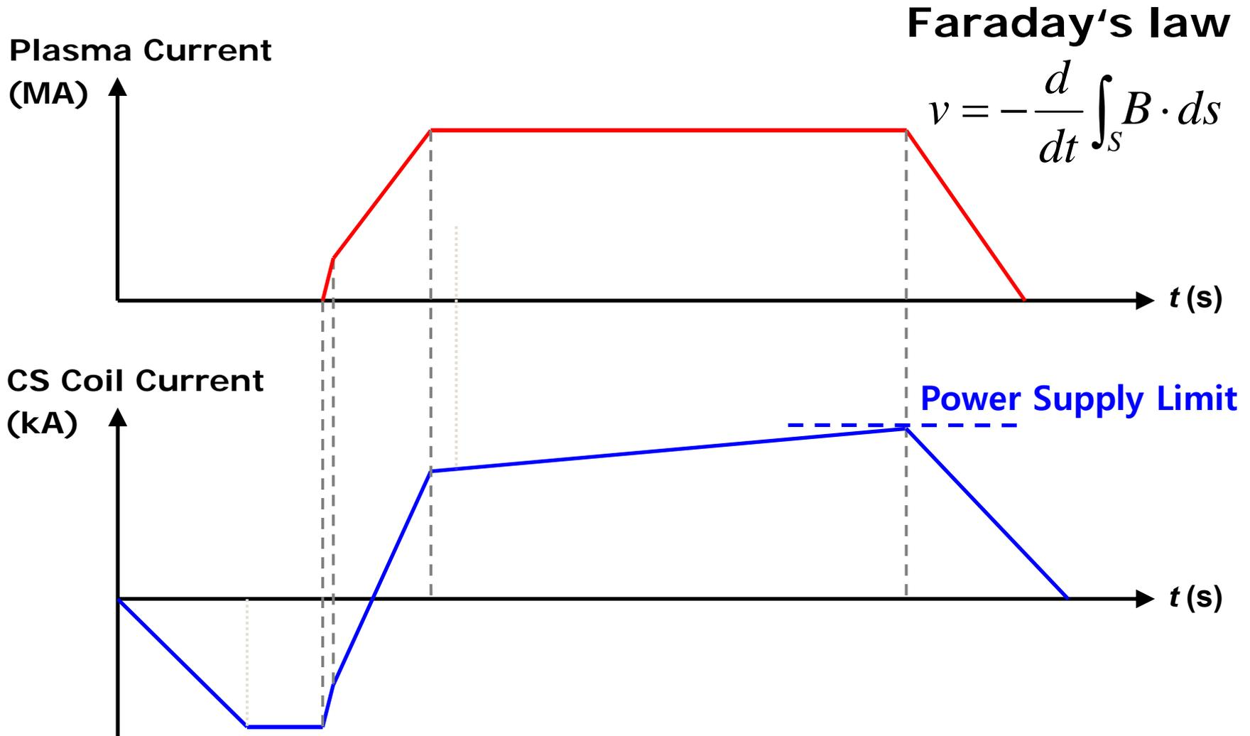
**Inherent drawback of Tokamak!**
