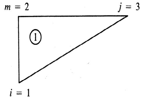
$$[B] = \frac{1}{2A} \begin{bmatrix} \beta_i & 0 & \beta_j & 0 & \beta_m & 0 \\ 0 & \gamma_i & 0 & \gamma_j & 0 & \gamma_m \\ \gamma_i & \beta_i & \gamma_j & \beta_j & \gamma_m & \beta_m \end{bmatrix}$$
