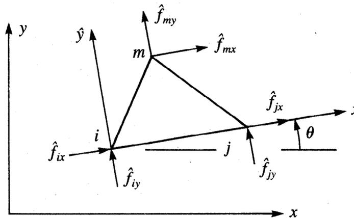
A triangular element with local coordinates system not along to the global coordinate system
