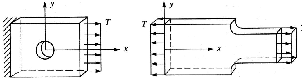
plane strain: The strain state when normal strain  $\epsilon_z$ , which is perpendicular to the plane  $x$ - $y$ , and shear strain  $\gamma_{xz}$ ,  $\gamma_{yz}$  are both zero.
