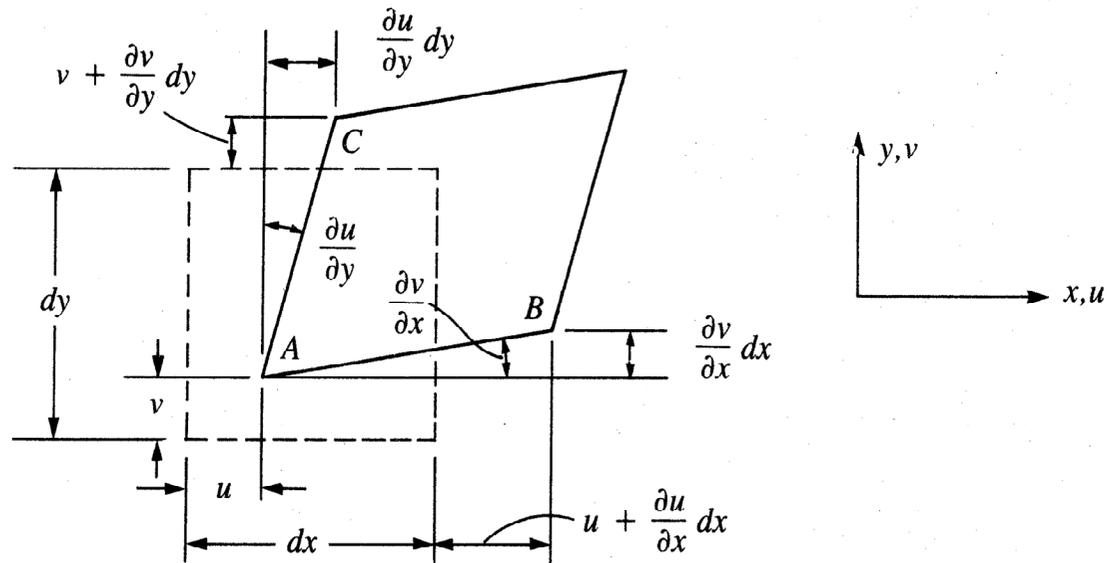
Displacement and rotation of plane element  $x - y$
