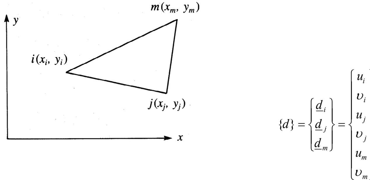
Considering a triangular element, the nodes  $i, j, m$  are notated in the anti clock wise direction.
