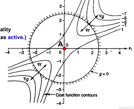
CASE #1: u=0 (The inequality constraint is considered as inactive at the solution point.)
