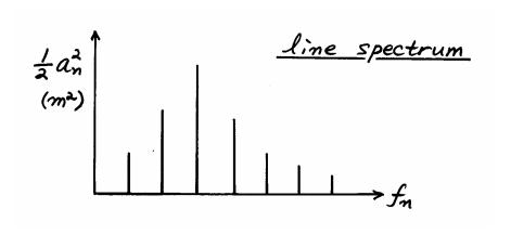
Real sea waves → infinite number of frequency components
