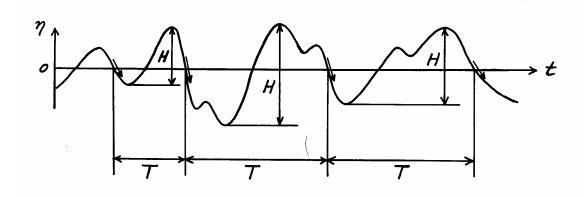
Statistically, zero-upcrossing and zero-downcrossing are equivalent if the wave record is long enough. But zero-upcrossing is more commonly used.
