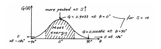
Intuitively, G = 0 for  $-180^{\circ} \le \theta \le -90^{\circ}$  and  $90^{\circ} \le \theta \le 180^{\circ}$ .
