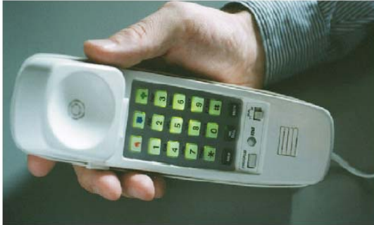
Fig. 1.7. AT&T telephone set ("Trimline" model) with the dial pad illuminated by two green N-doped GaP LEDs. The illuminated dial pad was one of the first applications of green GaP:N LEDs.
