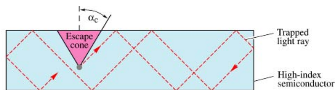
Fig. 6.3. Illustration of "trapped light" that cannot escape from a cube-shaped semiconductor for emission angles larger than \alpha_c due to total internal reflection.
