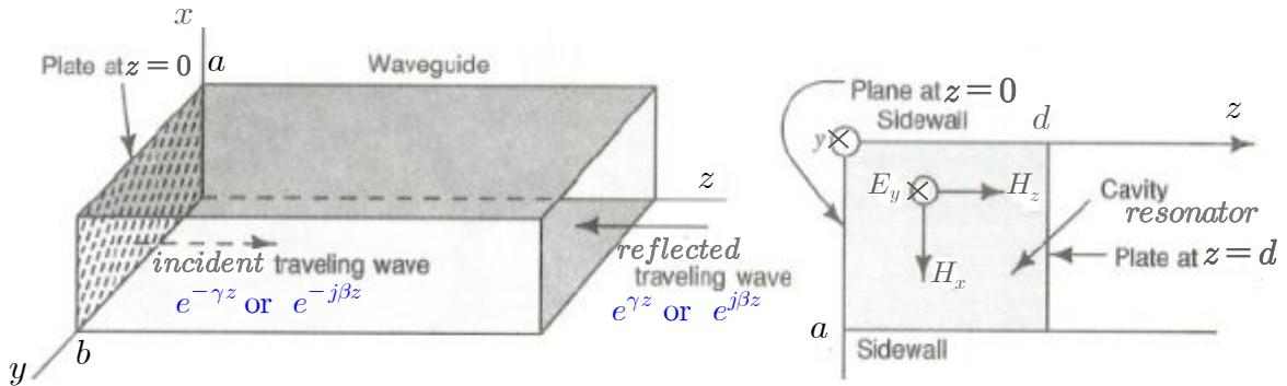
Choose the *z*-axis as the reference direction of propagation, then there exist *standing waves* in  $0 \leq z \leq d$  by incident and reflected TE or TM waves in the cavity.
